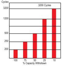
Number of cycles vs. depth of discharge at +20°C discharge with 20 hour rate
