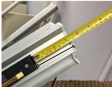
END CHARGING POINTS CAN NOT BE CLOSER THAN 2 3/4" FROM THE END OF THE RAIL
