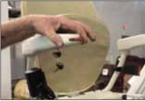
Using the arm switch , move the unit down the rail approximately 1 foot.
